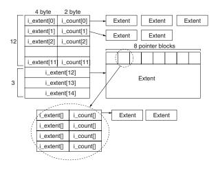
Fig. 2. i-node structure of HERMES file system
