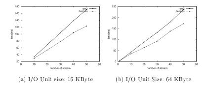
Fig. 4. Scalability Test: I/O latency of the streaming operation
